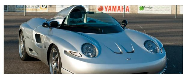
Evolved from the Classic Porshe 911, The W3 Triposto Features include a Kevlar and Fiberglass Composite Body, Push Button Parking Brake and Door Openers, Porsche 3164c.c. 252hp Engine, 5 Speed Transaxle, Modular Racing Wheels, Clamshell Instrument Pod, Road Speeds up to 165mph. This vehicle is so much more than just a fancy car, it's the pinnacle of engineering excellence combined with the greatness of pure imagination. It's designed to elevate and inspire the future automotive development.
